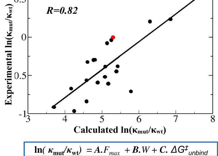
A, B and C are the slopes obtained from the linear fit between the exponential aggregation rate and the rupture force, work and unbinding free energy barriers, respectively
