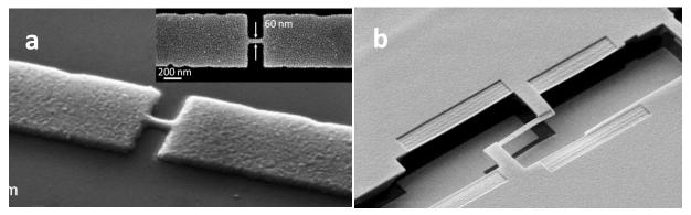
*Fig.3. SEM photos of the nanostructures* routinely obtained in my lab: (a) Aluminum nanobridge (b) E-beam defined PMMA/MMA mask for Al/AlxOy/Al tunnel junction (images taken at an angle).
