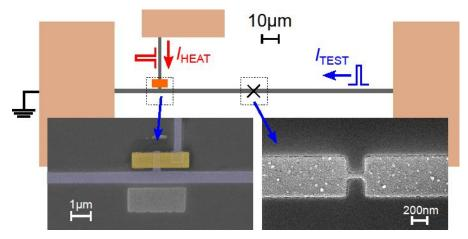
**Fig.12.** Layout of the sample for studying the dynamics of hot electron diffusion at miliKelvin temperatures. It consists of resistive copper island (SEM photo to the left) and a remote temperature sensor (aluminum nanobridge). A short heating pulse  $I_{HEAT}$  creates hot electrons which start diffusing towards thermometer along superconducting nanowire. The test pulse  $I_{TEST}$  is launched with time delay and probes temperature of the bridge (**Fig.13**).
