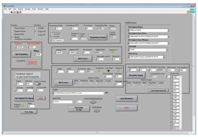
**Fig.23.** Front Panel of the **LabView acquisition program for performing switching measurements** on Josephson junctions developed over recent years by me. All data presented in publications **H1-H5** were acquired with that software being extended in time.
