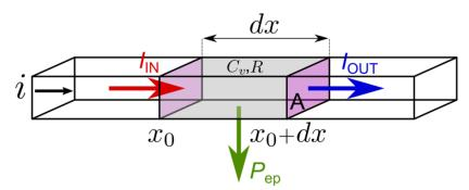
Fig.17. The graphical representation of energy conservation in a small volume Adx.
