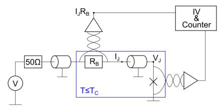
**Fig.5.** A simplified electrical circuit used in my laboratory to probe a junction with current pulses. It allows also to measure current-voltage (IV) characteristics of the junction (X in the figure). A counter (oscilloscope) records number of switching events observed as a voltage pulses V<sub>J</sub> developing on the junction.  $R_B$  is a bias resistor for monitoring the current sent to the junction I<sub>J</sub>. V stands for Arbitrary Waveform Generator (AWG) with 50  $\Omega$  output.
