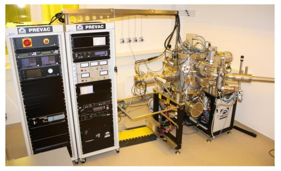
*Fig.21. Electron-beam evaporator with ion gun. Base vacuum* 2\*10<sup>-9</sup>*mBar (without annealing). The system is compatible with multi-angle e-beam lithography.*
