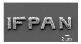
Fig. 9. Selective area growth of GaN NWs on a-Al<sub>x</sub>O<sub>y</sub> nucleation layer with SiN<sub>x</sub> mask. Figure from [H4].
