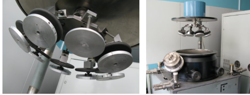
FIGURE 3.2: ion-beam sputtering system. Left — rotating placeholders; right — deposition camera with wide-aperture ion source.
