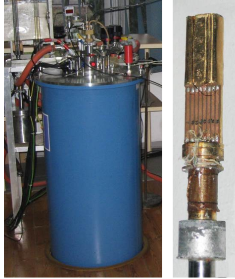
FIGURE 3.4: left — "Oxford Cryogenics" system with superconducting magnet; right — insert for magnetoelectric measurements.
