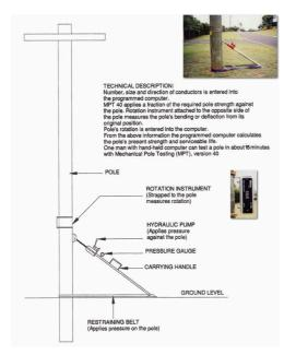
Figure 22: Outline of the Mechanical Pole Testing method (MPT) for electric power poles. [Deuar Pty. Ltd.]
