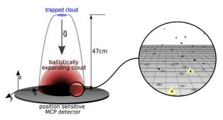
Figure 14: The experimental setup in Palaiseau. (Diagram as in [1]).
