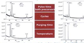
In our experiment we varied pulse time of both (water and diethylzinc) precursors, purging time, number of cycles and temperature. We observed changes in crystallographic orientation.
