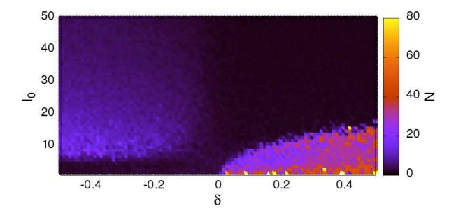
**Rysunek 1** We investigated numerical model of 1D stepped crystal surface under external current. We showed that step bunching emerges for the two directions of the current  $\delta$ . There is a narrow range of the initial terrace width 10 (miscuts), where the instability is observed for step up ( $\delta$ <0) and step down ( $\delta$ >0) directions of the drift.
