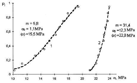
Fig. 4. Strength distributions for the abrasive materials: curve 1 is for the standard silicone carbide material, curve 2 is for the material doped by ultradispersed admixture.
