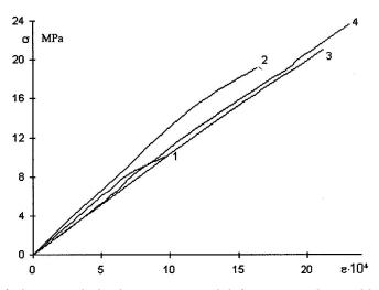
Fig. 3. Diagrams of silicone carbide abrasive material deformation, obtained by the formulae (4) and (5). Curves 1 and 2 represent standard material, the samples of which displayed correspondingly the minimum and maximum strength, curves 3 and 4 — the same for the material doped by the ultradispersed admixture.
