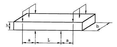
Fig. 1. 4-point system of beam loading.
