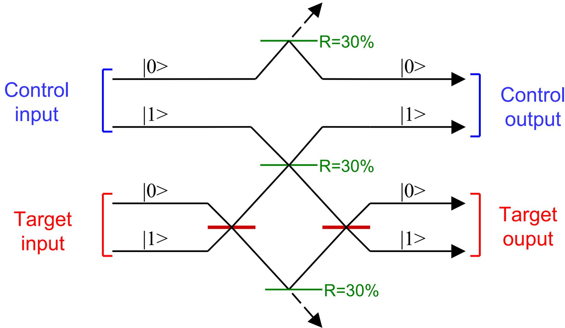
When **control output** and **target output** clic in coincidence (probability  $1/9$ ), the CNOT gate is realized.
