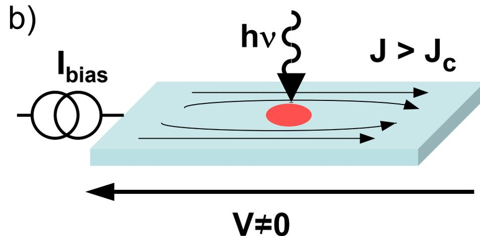
Superconductivity is suppressed by the absorption of a photon (thermalisation time: 20 ps)
