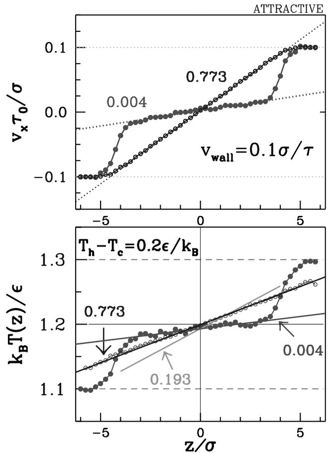
FIG. 3. Top: Velocity profiles in Couette flow for various  $\rho$ , in the narrowest channel with attractive walls; the upper and lower walls move with velocities  $\pm 0.1\sigma/\tau_0$ , respectively. The slip length for the high  $\rho$  case is  $-1.7\sigma$ . Bottom: The temperature profile in the thermal slip problem. The open and closed circles correspond to  $\rho = 0.773$  and  $0.004\sigma^{-3}$ , respectively. For  $\rho = 0.193\sigma^{-3}$ , only the central slope is indicated.
