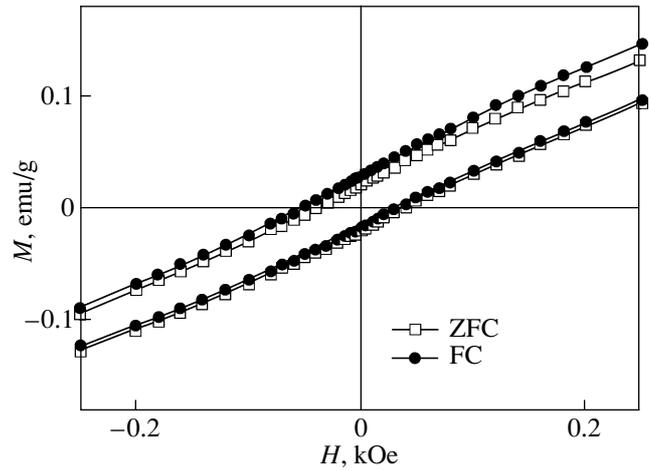
**Fig. 3.** Central part of the hysteresis loop of  $\text{ZnGeAs}_2$  sample with 3.5 wt. % Mn, which was measured at 5 K in a magnetic field from +0.6 to –0.6 kOe. We readily see the loop for the sample cooled to 5 K in a magnetic field of 0.6 kOe to shift along the  $H$  axis, whereas the loop measured in zero field is symmetric.
