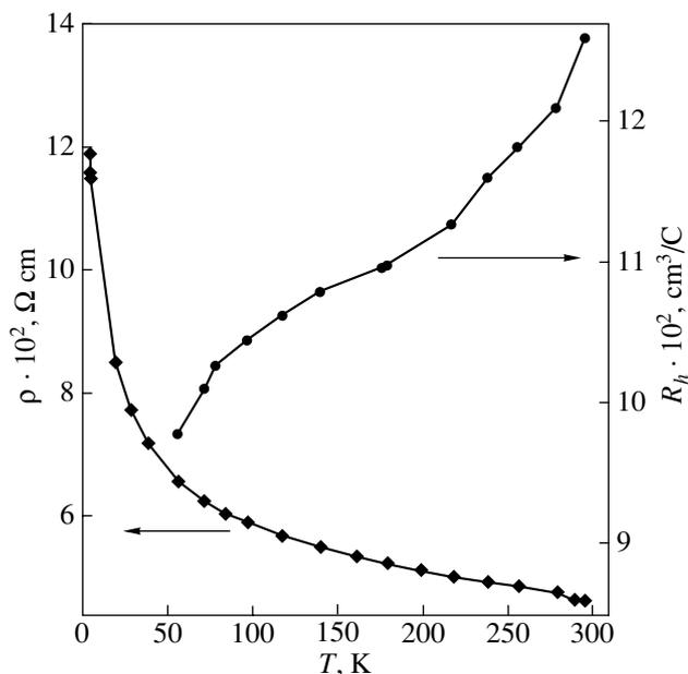
**Fig. 5.** Temperature dependence of the electrical resistivity  $\rho$  and the normal Hall coefficient  $R_H$  for the  $\text{ZnGeAs}_2$  sample with 1.5 wt. % Mn.
