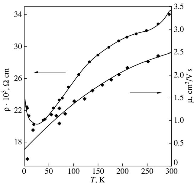
**Fig. 6.** Temperature dependence of the electrical resistivity  $\rho$  and the hole mobility for the  $\text{ZnGeAs}_2$  sample with 3.5 wt. % Mn.
