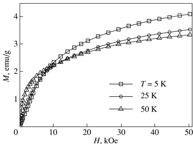
**Fig. 4.** Magnetization isotherms of the  $\text{ZnGeAs}_2$  sample with 3.5 wt. % Mn at different temperatures. Each curve was measured after the sample had been cooled to 5 K in a zero magnetic field.
