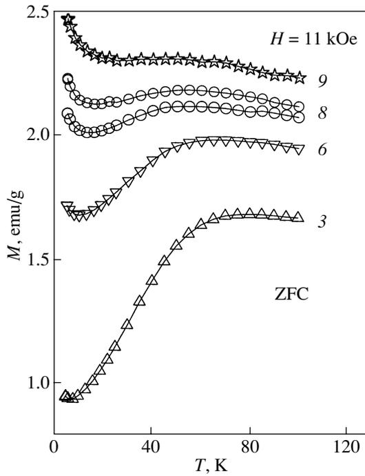
**Fig. 2.** Temperature dependence of the magnetization  $M$  for the composition  $\text{ZnGeAs}_2$  with 3.5 wt. % Mn in different magnetic fields in the temperature range from 5 to 100 K. Each curve was measured after the sample had been cooled to 5 K with no magnetic field.
