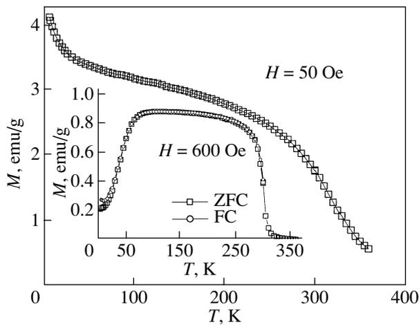
**Fig. 1.** Temperature dependence of the magnetization  $M$  for the composition  $\text{ZnGeAs}_2$  with 3.5 wt. % Mn in magnetic fields of 50 kOe and 0.6 kOe (inset). The ZFC curve: the sample was zero-field-cooled from 400 to 5 K, after which its magnetization was measured under heating. The FC curve: the sample was cooled in a field of 0.6 kOe from 400 to 5 K with parallel measurement of its magnetization.
