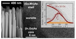
Figure 1. Electron microscopy images: left panel whole stack with NW axes oriented along D001] direction and side facets of (11-20) rientation. On average, the NWs have iameters of about 70 nm and lengths of up to  $\mu$ m (see Fig.1). Magnetic properties of NWs ensemble were
