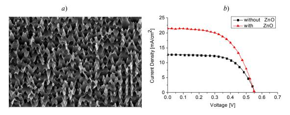
Figure 1: a) SEM image textured surface of ZnTe, b) Illuminated current–voltage characteristics for n-CdTe/p-ZnTe heterojunctions with and without ARC.
