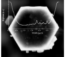
Fig. 1. *CL* map of the upper surface of ZnO nanorod obtained from solution of pH=7.
