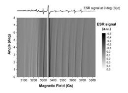
Fig. 1. Angle dependence of ESR spectrum of graphene with NaCl particles and cross-section for magnetic field perpendicular to the graphene surface.
