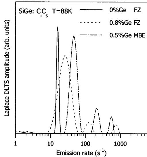
FIG. 16. The Laplace DLTS spectra of the  $C_i-C_s$  pair observed in the FZ silicon (solid line), FZ SiGe (0.8% of Ge) (dashed line), and the MBE-grown strained SiGe (0.5% of Ge) (dotted-dashed line) samples (Ref. 62).
