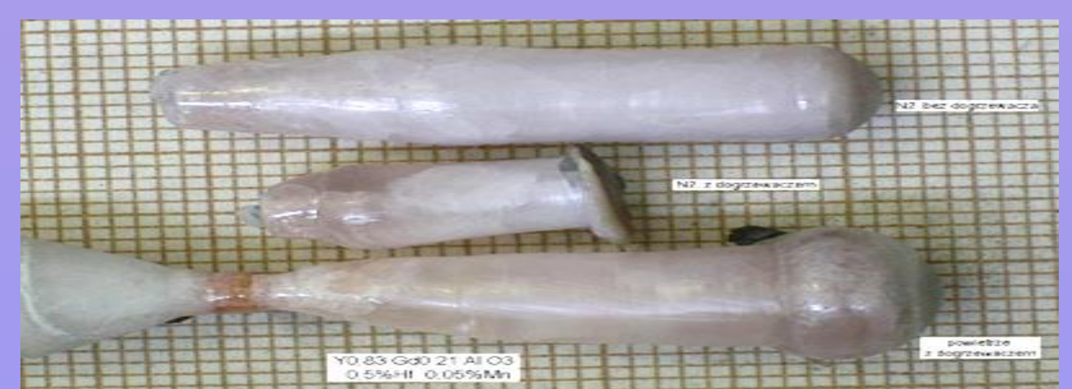
Figure 6. Single crystals grown in an optical furnace by zone melting
