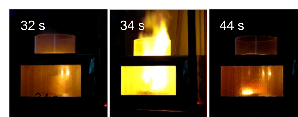
Combustion synthesis in a microwave oven over time: 32s, 34s, 44s.
