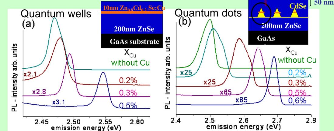
**Figure 2.** Normalized photoluminescence (PL) spectra from various samples containing (a) (Zn,Cd)Se:Cu QWs embedded in ZnSe and (b) CdSe:Cu/ZnSe QDs. Cu-concentration is controlled by Cu flux. The normalization factor is given for each spectrum, which indicates a significant quenching of the luminescence in the presence of copper. T = 5 K, excitation – 405nm
