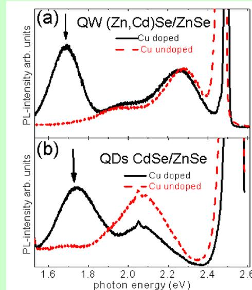
**Figure 3.** Comparison of the optical emission from Cu-doped and undoped structures, which leads to the identification of Cu-related optical emission from (a) ZnCdSe:Cu quantum wells with Cu content of 0.2% and (b) CdSe:Cu/ZnSe quantum dots with Cu content of 0.3%. The arrows indicate the emission showing up in the presence of Cu dopants. T=5K, excitation with 405 nm and 474 nm laser for (a) and (b), respectively.
