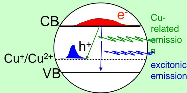
**Figure 1** Schematics of the Cu related emission when Cu level lies within the energy gap. The conduction band (CB) electron recombines with the hole strongly localized on Cu<sup>2+</sup> ion. e.g. Knowles KE *et al.* Chemical Rev. 116, 10820 (2016)
