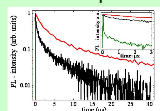
**Figure 6.** PL-decay times of the excitonic emission (green), Cu-related emission (red) in ZnCdSe:Cu QW with Cu content of 0.2% and Cu related emission from CdSe:Cu QDs with Cu content of 0.5% (black curve). Inset: close-up of PL at short delays. T = 5 K, excitation energy 405 nm.
