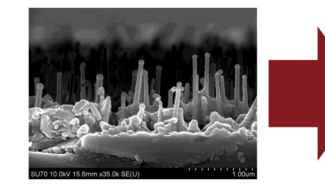
Deposition on the 3D surfaces (ZnO film on the cotton and nanorods.
