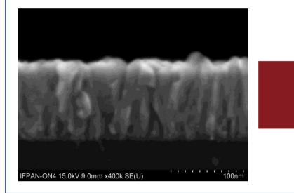
Precise thickness control (ZnO film)
