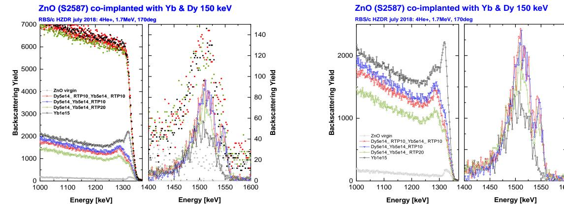
**Energy range 1000-1400 keV:** It has been found that, in case of Yb and Dy co-implantation, better recovery of the ZnO crystal lattice is achieved when one 20 min. annealing process is applied instead of two RTP processes, each after one implantation step (Dy or Yb). Energy range 1400-1600 keV: The RBS spectra show that similar
