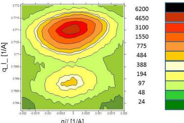
The ZnO/GaN/Al<sub>2</sub>O<sub>3</sub> films are grown with the c axis perpendicular to the surface (only two XRD reflections from 002 and 004 planes were observed). The FWHM of the 002 reflection is 158" (~0.04°), the same value was obtained for the GaN substrate.
