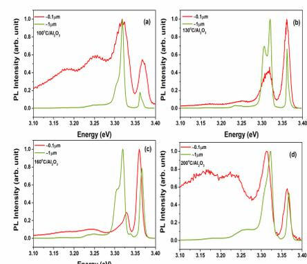
Fig.7. LT PL comparison of annealed thin and thick ZnO/Al<sub>2</sub>O<sub>3</sub> film at growth temperatures a) 100°C, b) 130°C, c) 160°C, and d) 200°C
