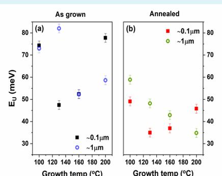
Fig.5. Urbach Energy for a) as-grown and b) annealed ZnO/Al<sub>2</sub>O<sub>3</sub> samples grown at different temperatures.
