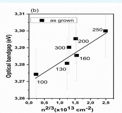
Fig.3. E<sub>g,o</sub> versus n<sup>2/3</sup> according to B-M effect for as-grown ZnO/Al<sub>2</sub>O<sub>3</sub> thin films.
