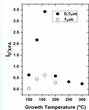
Fig.8. The relative intensity ratio of FA/D'X peaks versus growth temperature for annealed ZnO/Al<sub>2</sub>O<sub>3</sub> layers.
