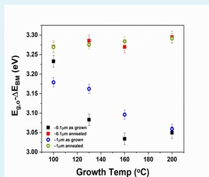
Fig.4. The corrected bandgap (E<sub>g,o</sub>-ΔE<sub>BM</sub>) versus growth temperature for thick and thin ZnO/Al<sub>2</sub>O<sub>3</sub> samples.
