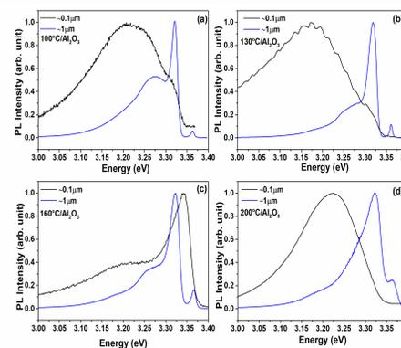
Fig.6. LT PL comparison of as-grown thin and thick ZnO/Al<sub>2</sub>O<sub>3</sub> film at growth temperatures a) 100°C, b) 130°C, c) 160°C, and d) 200°C
