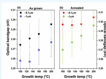
Fig.2. Optical bandgap for a) as-grown and b) annealed ZnO/Al<sub>2</sub>O<sub>3</sub> samples grown at different temperatures.
