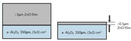
Fig.1. Schematic diagram of ALD process and ZnO/Al<sub>2</sub>O<sub>3</sub> thick and thin film
