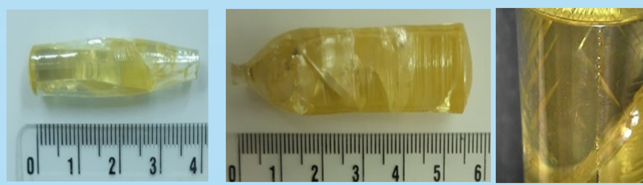
Pure LiNbO 3 single crystal (left) and doped with 0.5% at Pr
