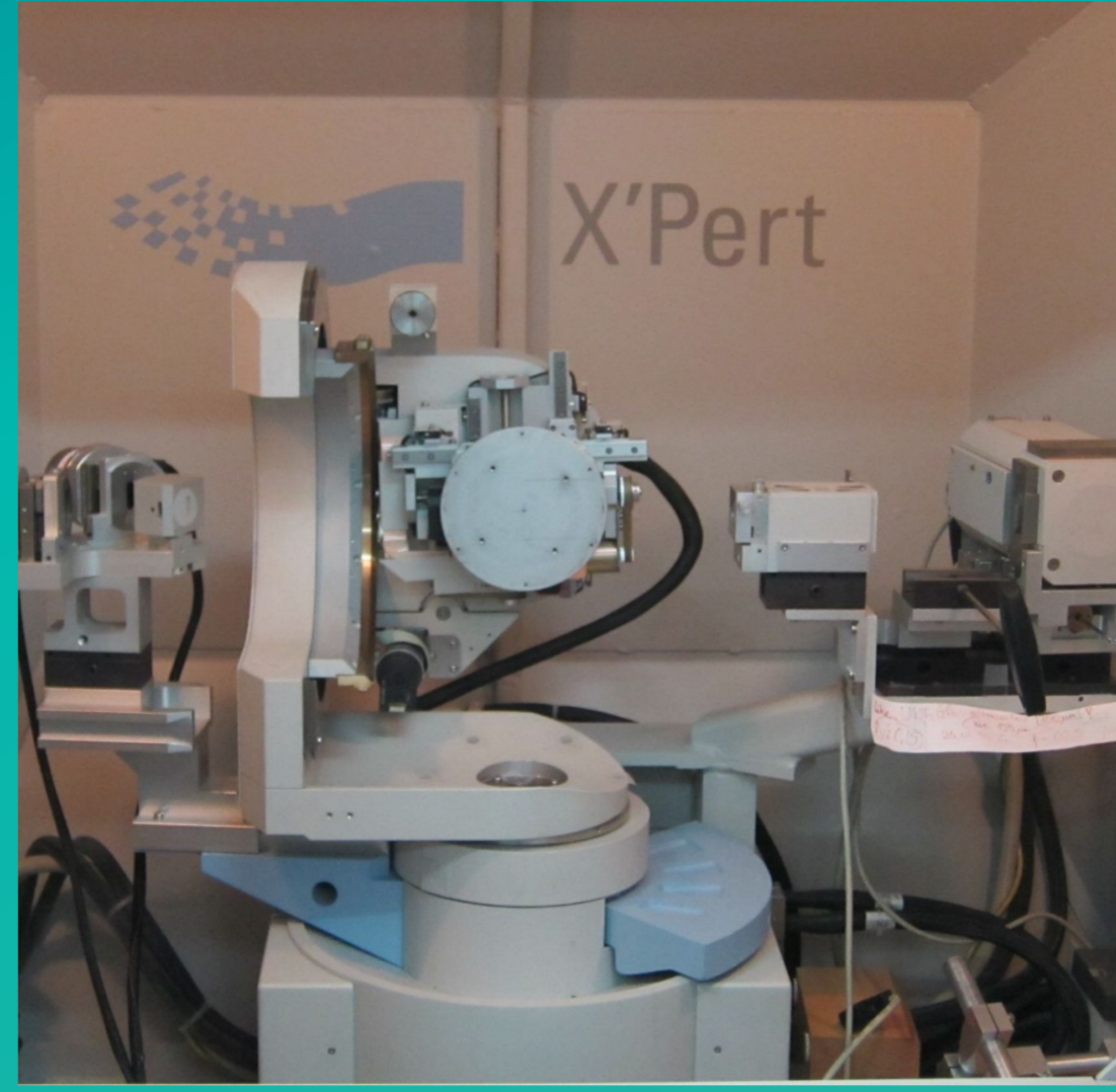
a high-resolution X-ray diffractometer with a 4-reflection Ge (220) monochromator and X-ray mirror, radiation - \text{Cu}_{K\alpha} and an analyzer in front of a proportional detector
