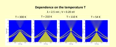
The gap closes at 110K. Below the band gap opens and the electronic band structure is inverted. Together with band gap also the gap in the Kramers point opens after decreasing the temperature.
