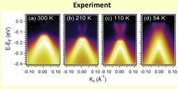
Rashba effect observed in ARPES maps of the MBE grown Pb054Sn046Te (111) epilayer topological crystalline insulator (TCI) with Bi doping of 0.25% at.
