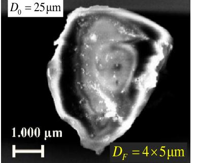
Nearly stable 3D SDS crystallised microobject
