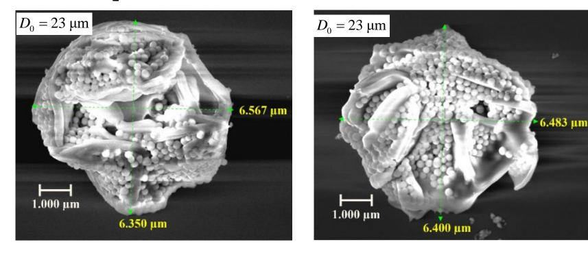
SDS/SiO<sub>2</sub> microobjects of nearly similar shapes from the same initial droplet size and composition
