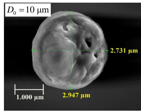
Smallest SDS/SiO<sub>2</sub> spherical microobject
