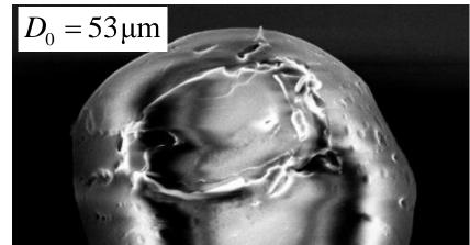
Formation of highly ordered spherical aggregates of silica nanospheres [1]
