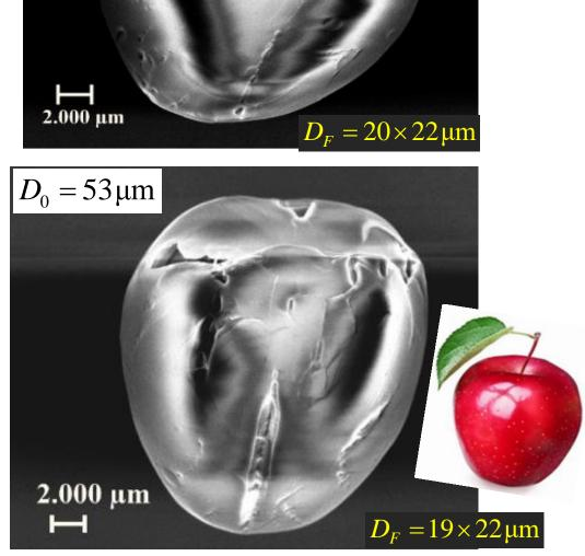
Micro-apple-like 3D SDS crystallised microobject
